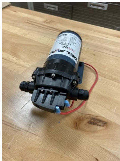
Figure 14: Pump connection fittings.
