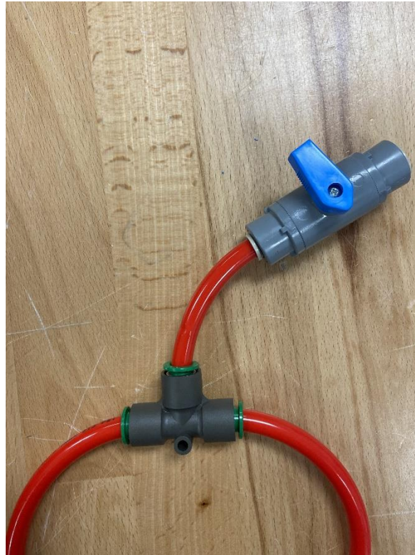
Figure 16: Joint and ball valve on supply line.
